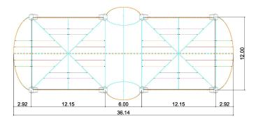
The ETFE sheet is printed with a silver coloured dot design, with the aim of improving interior comfort, while maintaining the transparency of the covering. In addition, cables are added to reinforce the membrane at the most demanding points.
